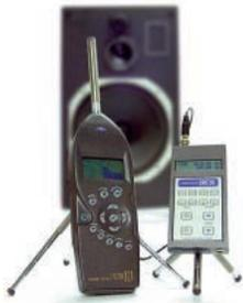
The SRC20 digital signal generator is ideal for laboratory and field tests. It provides extremely stable and repeatable sine, swept sine, pink and white noise signals for reverberation measurements, vibration excitation, audio system equalization, and electronic measurements. With the 824-RTA triggering capabilities, you have a very portable system where source and analyzer do not have to be linked by cables.
